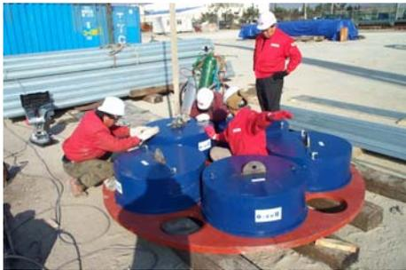
Assembly of the 5x 870 mm O-cell arrangement
