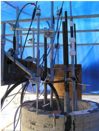
Test Instruments at Pile Head
